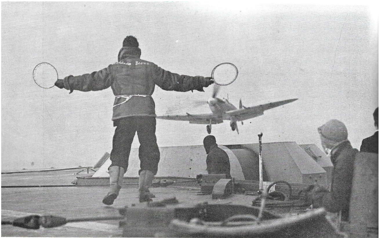
THE GREAT DAY. Landing on a carrier after shore training is finished is a great moment. The Deck-Landing Control Officer guides the Seafire pilot in with his "bats."
